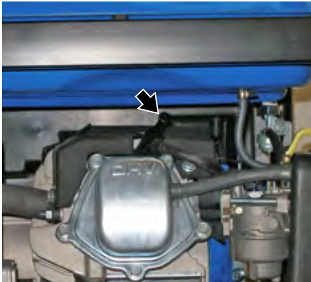
Figure 36 – Removal of Spark Plug Boot
