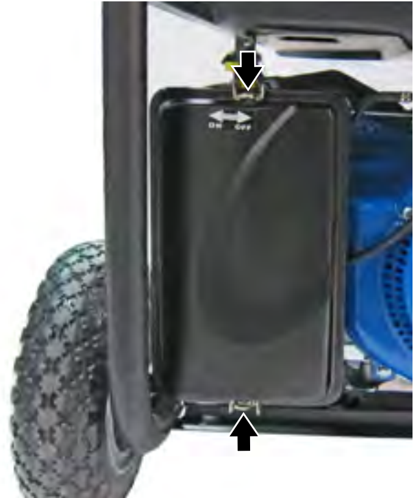
Figure 35 – Installation of Air Filter Cover
