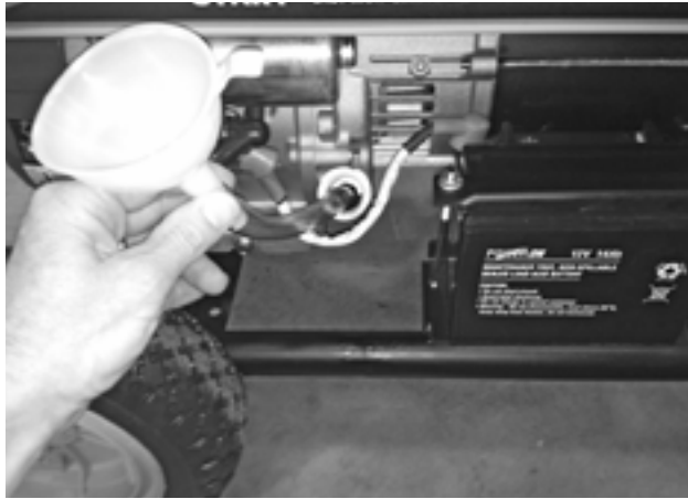
Figure 28 – Adding Engine Oil
