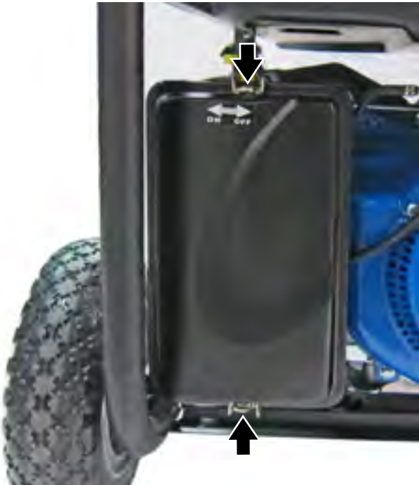
Figure 30 – Removing Air Filter Cover
